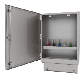
The FFGCC-A1 Series Generator Connection Cabinets offer quick connection to a mobile generator allowing temporary power to be received quickly and safely. They can be penetrated from the side, back or top to allow for facility wiring. These units are equipped with colour coded Camlock receptacles allowing for easy connection. Assemblies are available up to 1200A and are ETL-certified.
